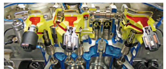
The fully automatic valve control system reduces CO 2 -emission by up to 25 per cent.
